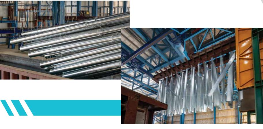
Maximum Throughput Galvanizing Furnace 20 To/h
